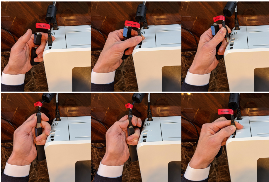
Figure 12: Installing Malware in the Polling Place. An attacker can install vote-stealing malware on the ICX by attaching a small USB device for under two minutes. This sequence shows me reaching behind the printer, unplugging the cable that leads to the BMD, and connecting the device to the end of the cable. This can be accomplished in seconds and does not require breaking any tamper-evident seals. It could potentially be carried out surreptitiously by a voter.
